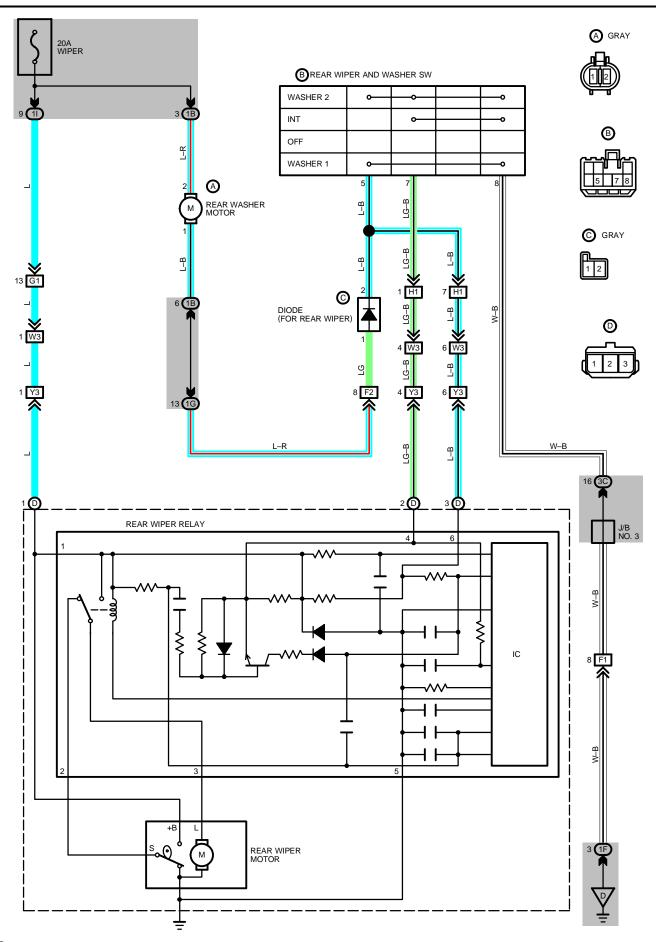
WHEN THE IGNITION SW IS TURNED ON, CURRENT FLOWS THROUGH THE WIPER FUSE TO TERMINAL 1 OF THE REAR WIPER RELAY, TERMINAL +B OF THE REAR WIPER MOTOR AND TERMINAL 2 OF THE REAR WASHER MOTOR.
